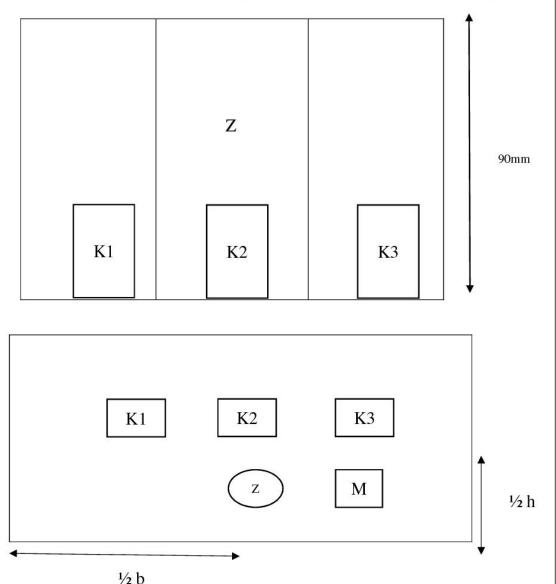
Z = TENSILE SPECIMENS (LONGITUDINAL DIRECTION) K1, K2 & K3 = IMPACT SPECIMENS
