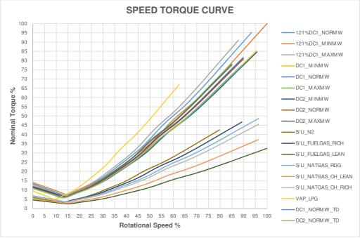
The motor is provided with VFD in order to realize different operating conditions as specified by the customer. These are indicated by the curves as shown above.
