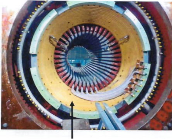
For support and consolidation of the overhang structure of large size TG (above 500 MW ratings).
