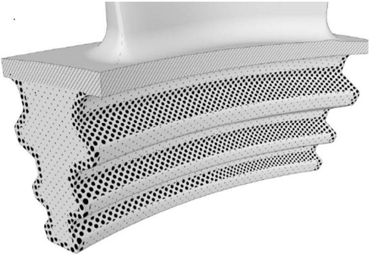
Figure 1: Peening of the transition to face area
