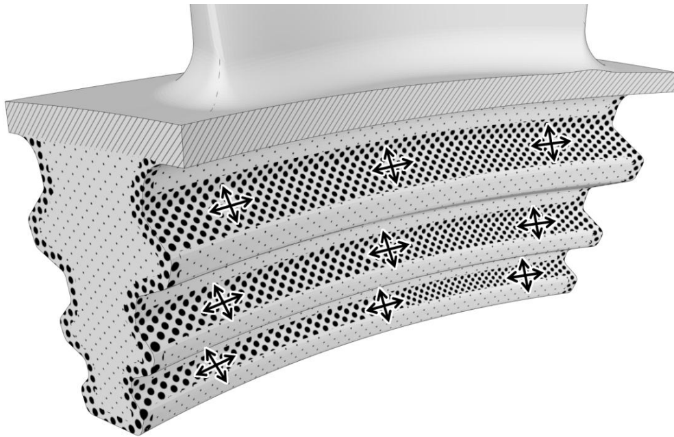
Figure 4: Positions of surface roughness measurements at the bearing flanks. Measurement shall be carried out on both sides (suction side and pressure side).
