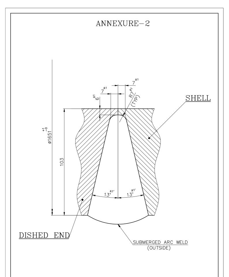
TYPICAL CIRSEAM WELD JOINT EP STYLE
