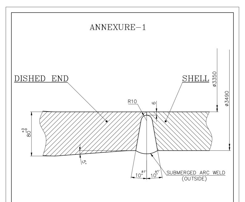
TYPICAL CIRSEAM WELD JOINT EP STYLE
