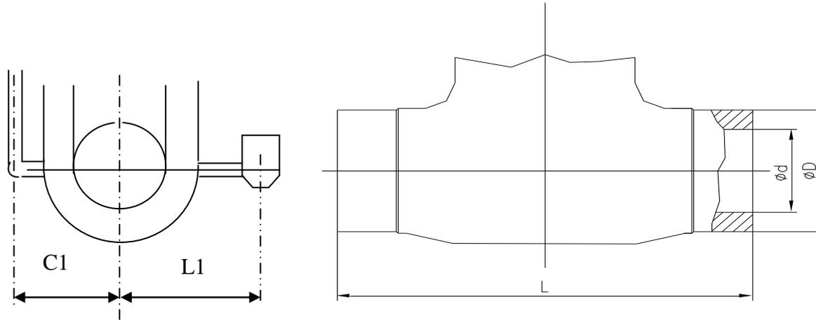
**Max C1 : 300 mm      Max L1 : 700 mm      (for 2” - 6” valves)**
