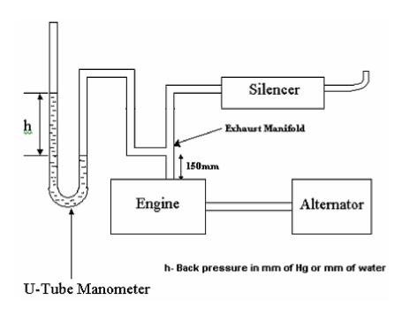
Back Pressure should be measured at 100 % loading condition
