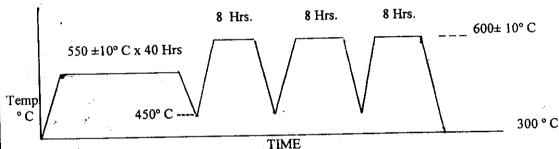
MAX. Rate Of Heating / Cooling = 30°C / Hr
