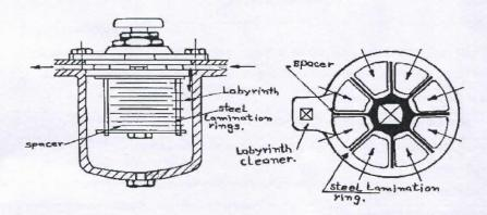
The oil to be filtered enters from outside and passes through the clearance between laminations. Impurities deposit on the edges. The filtered oil flow through the sector shaped holes of the laminations to the upper part of the filter pack and subsequently to the system.
