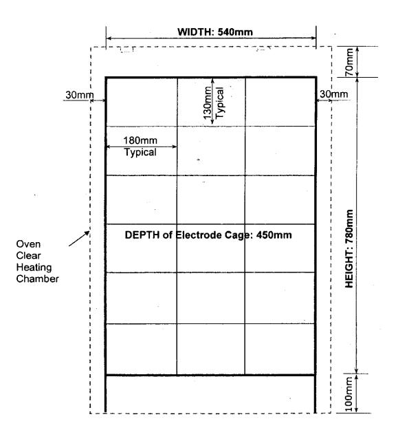
Depth of Oven clear heating chamber: 600mm
