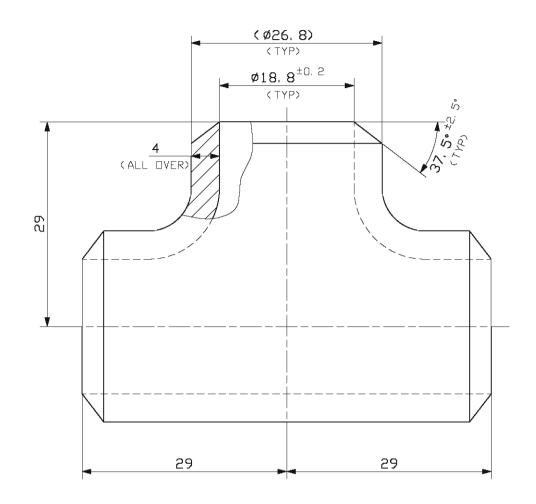
TOLERANCE IF NOT SPECIFIED SHALL BE AS BELOW (REFER IS 2102-m)
