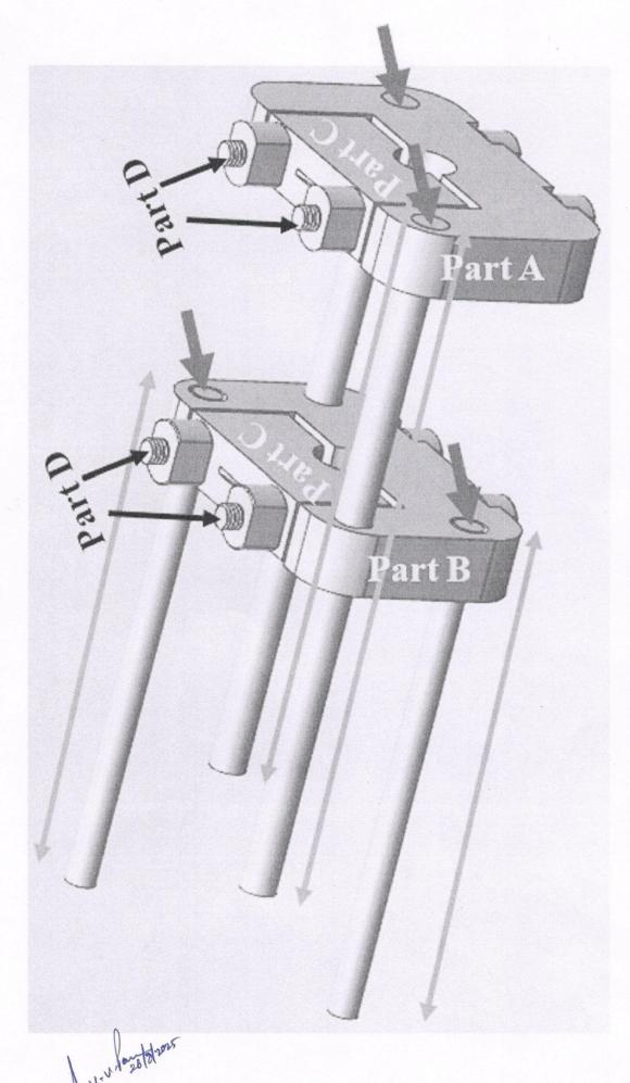
: Rod of diameter 5.9 mm and length 510 mm (+/-5% tolerance)
