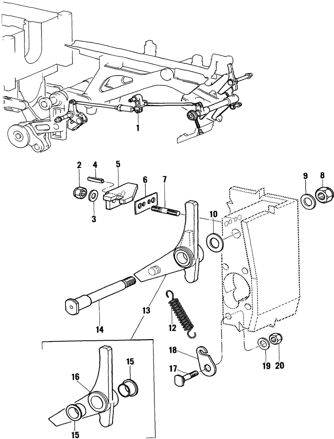
**Loading Tray Releasing Transmission**
