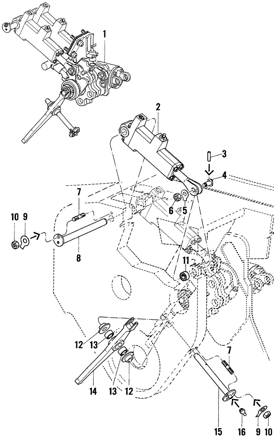
**Loader Drum Transmission and Actuator Cylinder**
