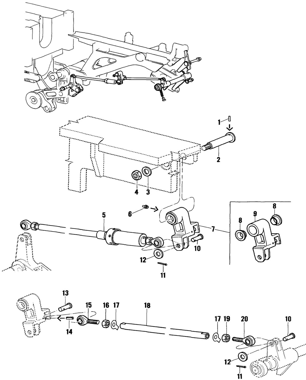
**Loading Tray Releasing Transmission**
