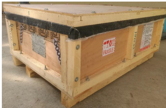
Fig. 1b : Typical bolted type construction of Box
