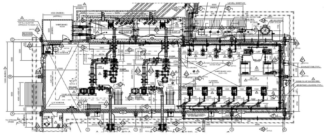
Layout of FA slurry Pump house
