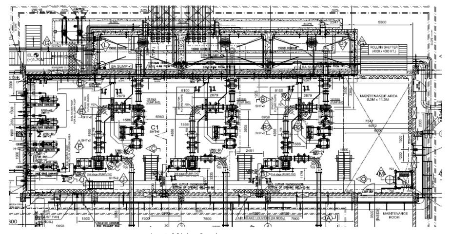
Layout of BA slurry Pump house
