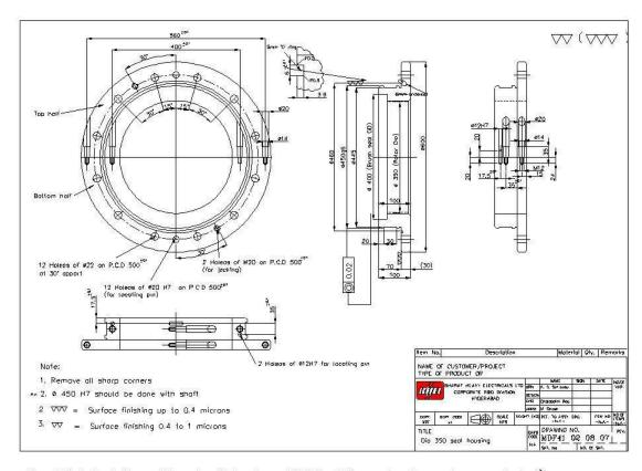
Brush & Labyrinth seal Housing (Brush seal OD & width can be changed as per design)
