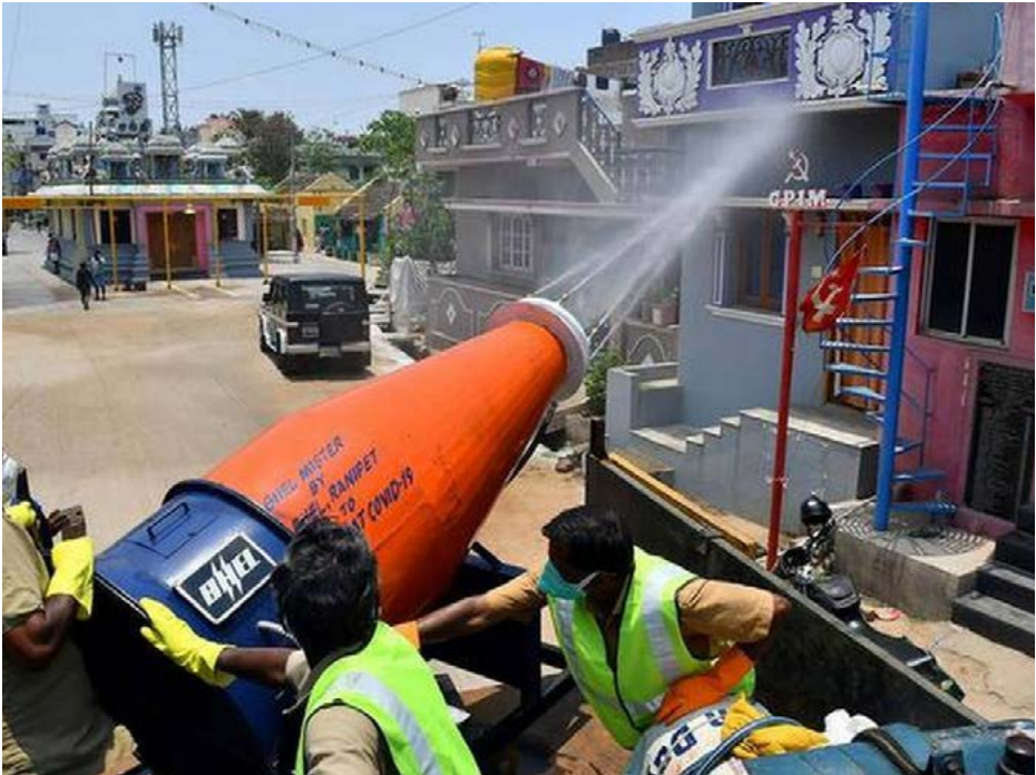
BHELMister developed by BHEL - a spray assembly for mass sanitisation, in action in Vellore, Tamil Nadu
