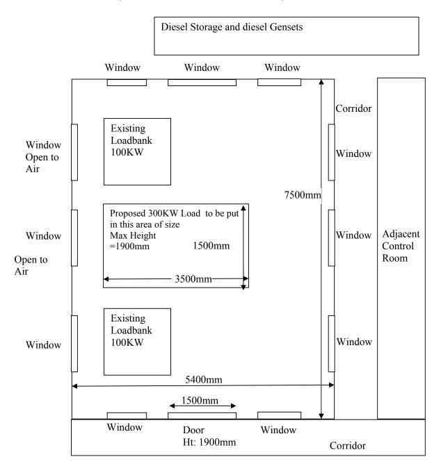
Figure1: Rough Sketch of Room Layout where loadbank is to be situated.
