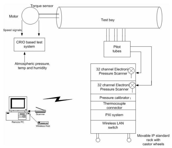
The requirement of the data acquisition system is to measure various parameters during the fan testing operation in BHEL and store the data in a remote PC and do various user defined analysis on the data and create a report as per user requirement.
