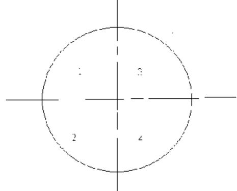
3 Green rupture test specimens according to EN 10291 (specimen 4 for reserve)
