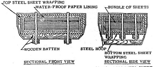
DETAILS OF PACKING FOR MAGNETIC STEEL SHEET
