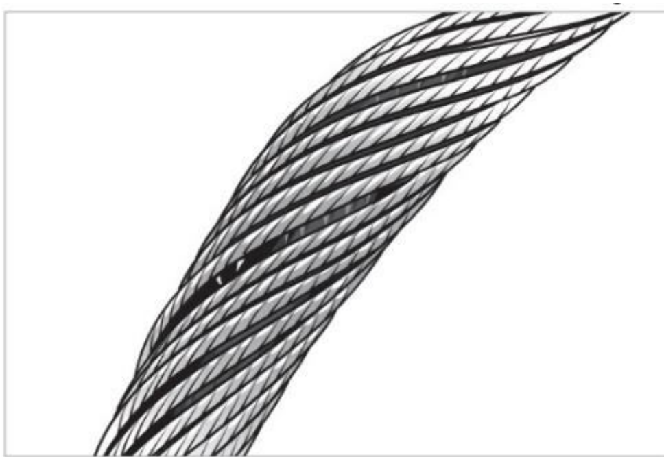
Birdcage or Basket/Lantern Deformation
