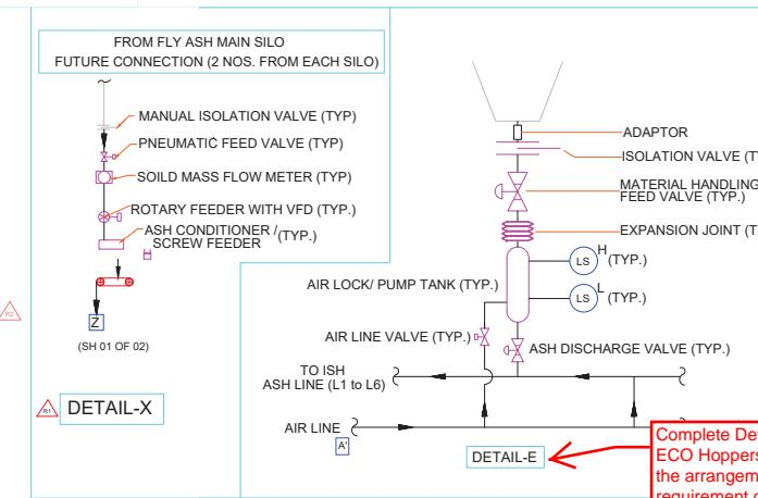
Complete Detail E is not applicable for ECO Hoppers. Below Expansion Joint, the arrangement shall be as per requirement of ECO Metallic Belt Conveyor.
