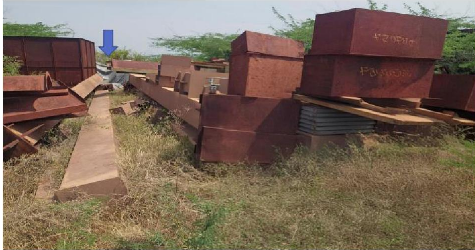
ID Rotor kept at Uppur site storage yard, Front area of around 75 meters to be cleaned and other material around 50 MT to be removed to make Cranes reach near ID fan Rotor for loading.
