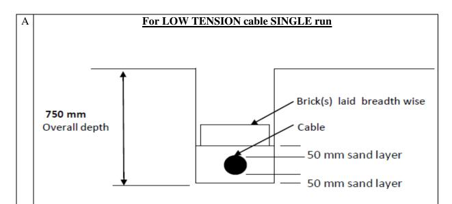
**For ONE run of cable**: The **trench should be excavated** to a depth, such that the cable will be laid at a **minimum depth of 750 mm** as shown above. Spread 50 mm deep layer of sand below the cable in trench, after laid the cable, also spread 50 mm deep layer of sand above the cable. Lay good quality bricks **breadth wise** only and cover the sand layer all along the cable / trench. Then complete the earth filling. The bricks shall be of good quality with size 100 mm x 75 mm x 225 mm
