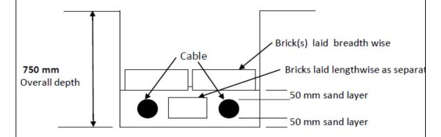
The cables should be laid in horizontal plane. The **trench should be excavated** to a depth and breadth, such that the cables will be laid at a **minimum depth of 750 mm in horizontal plane** as shown above. Spread 50 mm deep layer of sand below the cables. Lay the cables in horizontal plane & place **good quality bricks** in between **them <u>length</u>**
