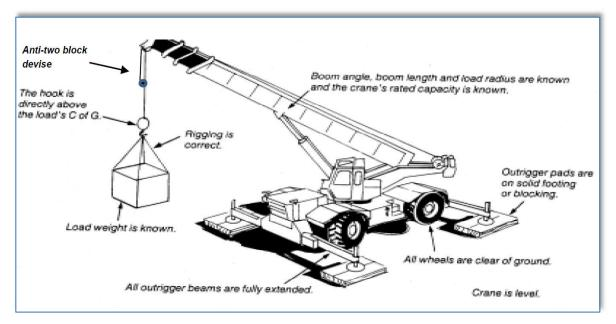
Fig. 5.2 Proper Crane Setup
