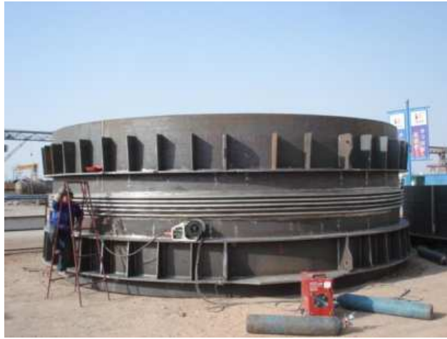
MSED Expansion Joint DN8000 Site Fabrication
