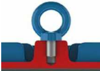
Correct tightening of the eyebolt
