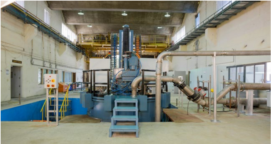
Unique High Temperature Spin Test Rig (HTSTR) established for testing of advanced materials for AUSC mission project
