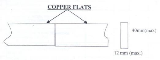
**NOTE**:-To be brazed by keeping inductor on top of butt joint of copper flats.
