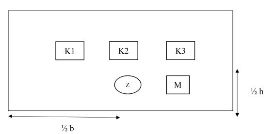
Z = TENSILE SPECIMENS (LONGITUDINAL DIRECTION) K1, K2 & K3 = IMPACT SPECIMENS
