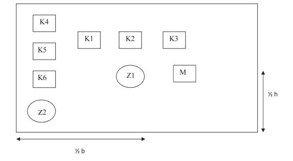
Z1, Z2 = TENSILE SPECIMENS (LONGITUDINAL DIRECTION) K1 TO K6 = IMPACT SPECIMENS M = METALLOGRAPHY SPECIMENS
