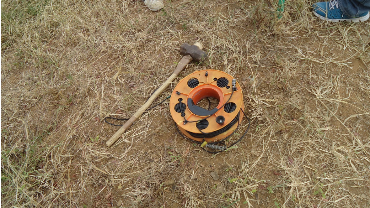
Photo: 17 Hammer with Trigger Winch & Cable
