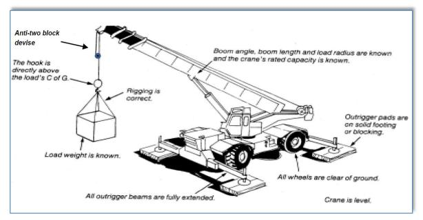
Fig. 5.2 Proper Crane Setup
