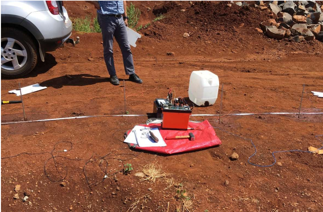
Figure 4 – Complete device: Terrameter, electrodes, battery and sets of cables
